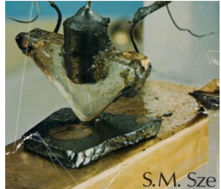
The first transistor, invented at Bell Laboratories 1947
