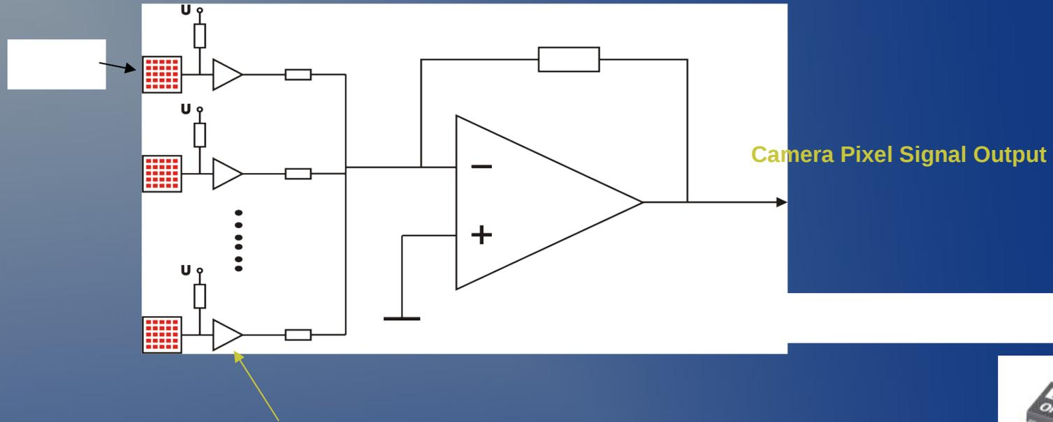
Fast transimpedance amplifier → currently developed at MPI
