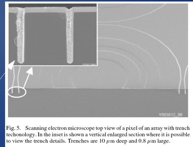
Fig. 5. Scanning electron microscope top view of a pixel of an array with trench technology. In the inset is shown a vertical enlarged section where it is possible to view the trench details. Trenches are  $10 \mu\text{m}$  deep and  $0.8 \mu\text{m}$  large.
