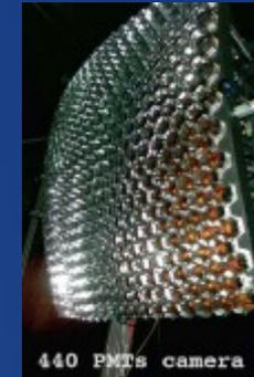
One AUGER fluorescence telescope
