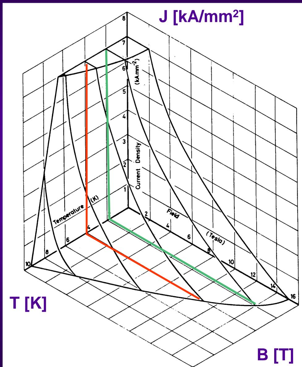
The superconducting state only occurs in a limited domain of temperature, magnetic field and transport current density
