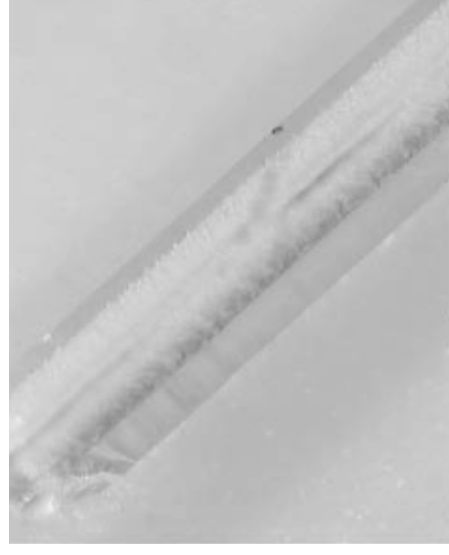
Cracks in the dielectric
